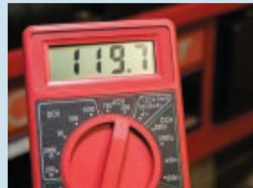
Check your generator's output regularly to ensure it's within a few percent of 120 volts. A simple electric multi-meter is what you need to perform this test.
