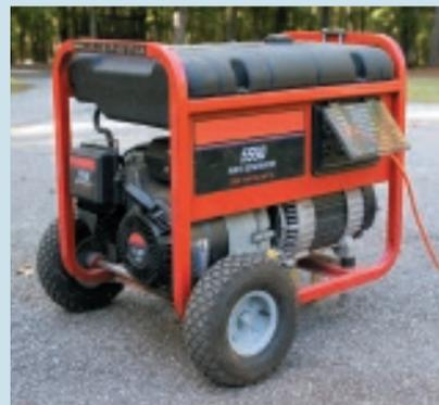
One of the features to consider when purchasing a generator is how you'll start it. The choices are manual (shown here) or electric where you simply turn a key. Once you have a generator, start and run it regularly to ensure the unit is ready when you need to press it into service.
